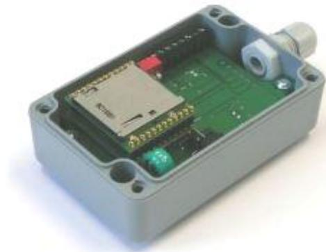
This Data Logger records analogue values from two 4..20 mA current loop interfaces. The values are sampled at an adjustable rate and stored into a file on the memory card together with a time stamp. The data are stored in a text format – which is easy to import into Excel or other analysis programs. Long term data acquisitions are possible due to SD card support of up to 16 GBytes. The interfaces are galvanically isolated to separate power supply and interfaces.
